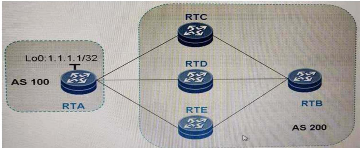
As shown in the figure, RTA belongs to AS 100 and has an EBGp neighbor relationship with RTC, RTD, and RTB is an IBGP neighbor of RTC, RTD, and RTE, and the four router all belong to AS 200.
