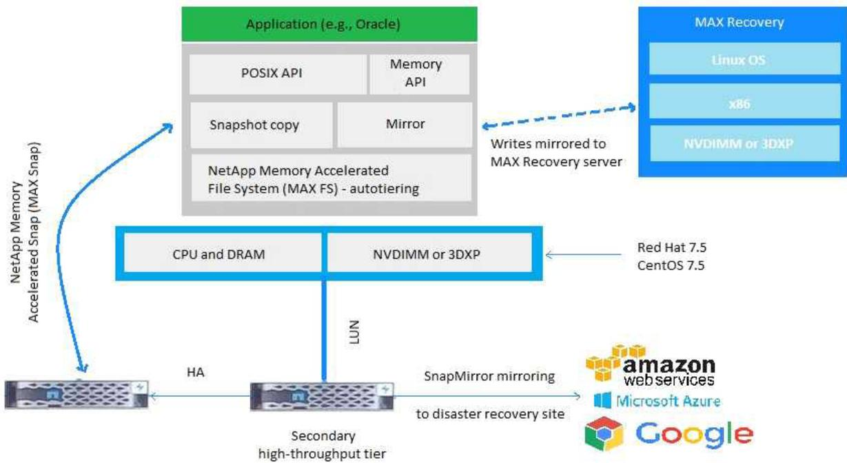
You have a requirement to serve LUNs with under 200 microsecond latency using local server lass memory. You also are required to use a shared SAN. Using MAX Data as shown in the exhibit, which two LUN access protocols are supported with this solution? (Choose two.)
