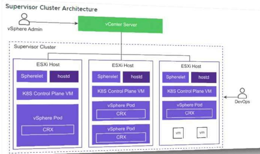
Spherelet is a kubelet that is ported natively to ESXi. It allows the ESXi host to become part of a Kubernetes cluster. Spherelet performs the following functions:
