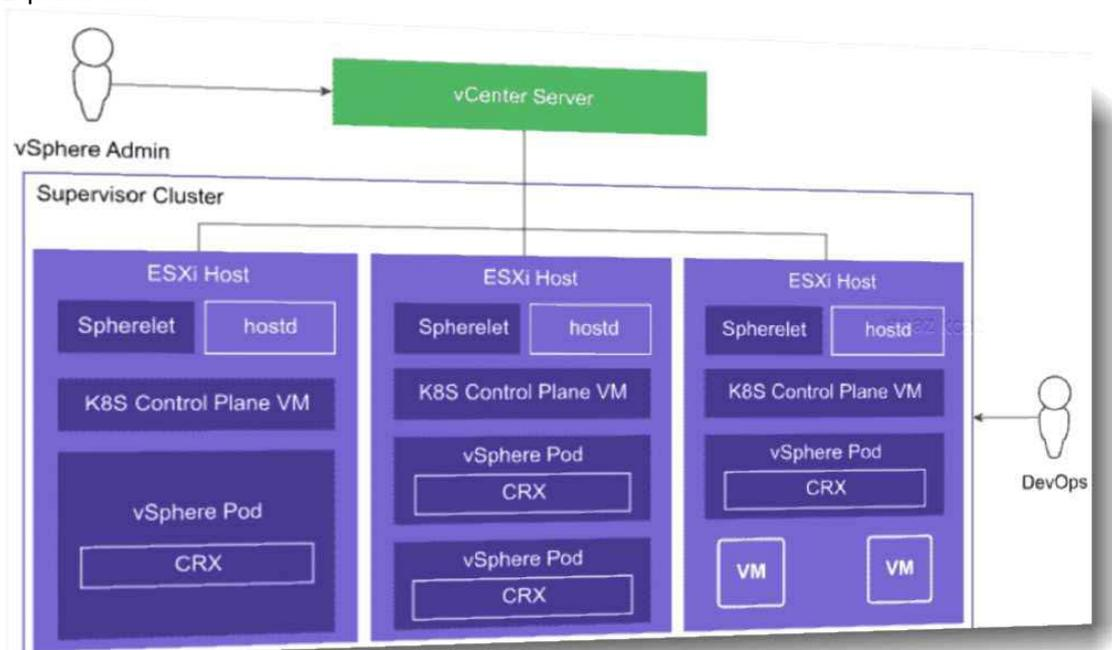
A vSphere Pod is a VM with a small footprint that runs one or more Linux containers. With vSphere Pods, workloads have the following capabilities:
