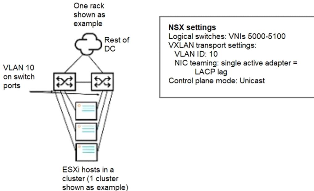
The exhibit indicates the customer NSX design and your plan for the connected ToR switches, which are ArubaOS-CX switches.
